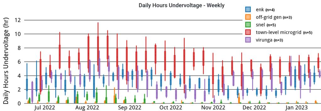
Figure 9: **IQR daily hours undervoltage over the past three months.** Town-level microgrids exhibit the most daily hours undervoltage of all the groups, typically, and the most variation. ENK and Virunga (both large, hydro operators) are also fairly unreliable, with sometimes more than four daily hours undervoltage. We define “under-voltage” as more than 10% below nominal, i.e. 198 V.
