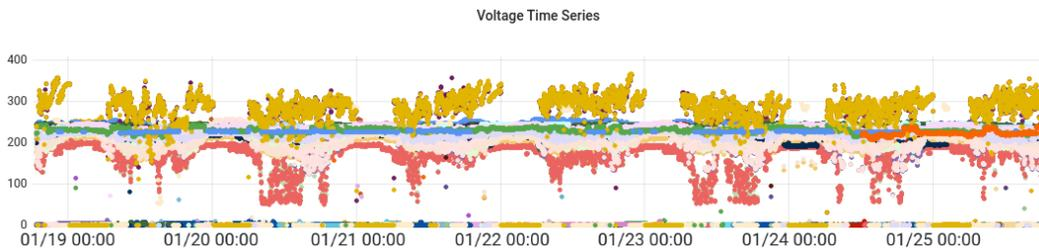
Figure 1: **One week of voltage data collected by PowerWatch sensors at 27 healthcare facilities in eastern Democratic Republic of Congo.** Each PowerWatch takes a measurement every two minutes of voltage magnitude, frequency and power state. Nominal voltage is 220 VRMS in the DRC. Outages and frequent voltage excursions from the nominal range, like those seen here, take a toll on sensitive equipment such as those in healthcare facilities.
