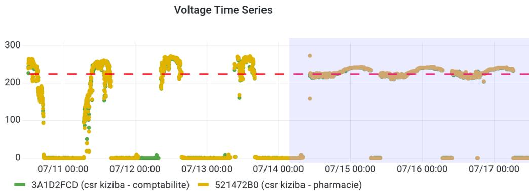
Figure 12: **Voltage before and after supply switch.** This high resolution voltage magnitude time series clearly shows the point where the CSR Kiziba HF transitioned from its own PV system to the solar minigrid provider Nuru on July 14, 2022 (shown with the shaded box). Voltage fluctuations improved after the connection and, although there continued to be nightly outages, these outages were shorter.
