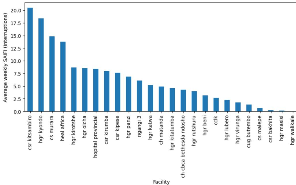
Figure 11: **SAIFI: Average Weekly Grid Interruptions.** Interruption frequency varies widely, from 20.5 interruptions per week, on average, at CSR Kitsambiro, to none at HGR Walikale, the off-grid facility on its own, new solar system.
