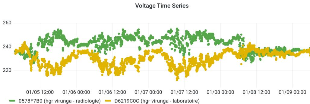
Figure 10: **Voltage recorded at two-minute intervals by the two sensors at HGR Virunga, one in the radiology room, and one in the lab, over the course of a few days in January 2023.** This anti-symmetry is persistent from when the facility was first instrumented. The X-ray technician told us the X-ray machine malfunctions, which could be caused by these large voltage deviations (frequently above 250 V).
