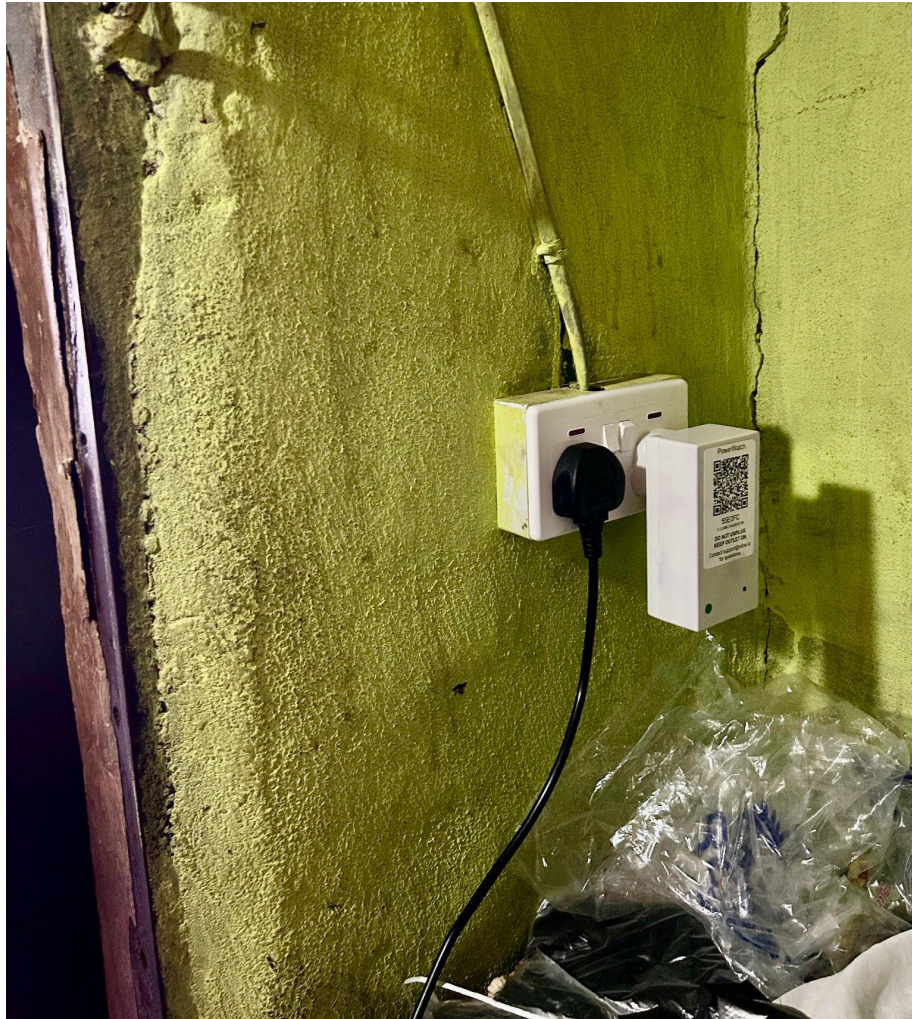
Figure 3: A GridWatch sensor plugged into a wall outlet at a grid-connected business in Freetown.
