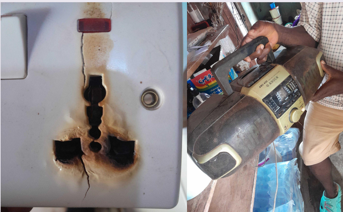
Figure 32: A wall outlet (left) and radio (right) were damaged by a voltage spike at three sampled businesses in Murray Town.
